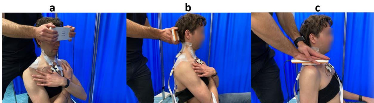
**Fig. 4** Experimental setup for high-density EMG-force tests. **a** Neck flexion contractions, **b** neck extension contractions and **c** shoulder shrug contractions (The images are original pictures taken by the team)
