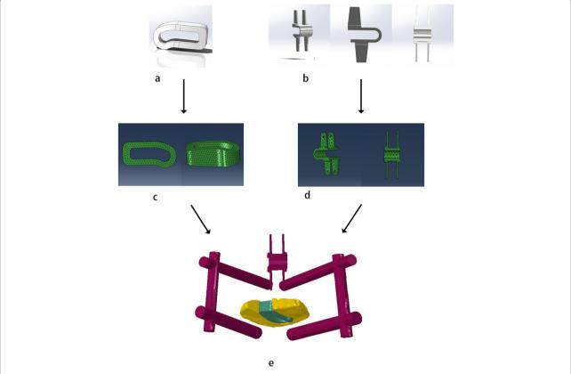
**Fig. 1** The process of establishing the internal implants models-from Constructing a geometric models of cage (**a**) and coflex (**b**) to finite element grid division (**c** and **d**), and to implants' commination (**e**) from Topping off model
