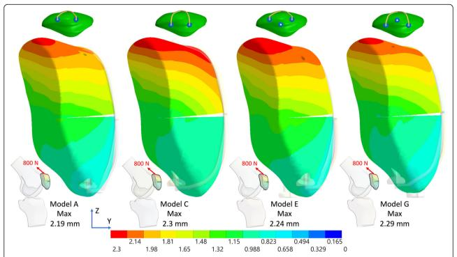
Fig. 3 Total displacement of the fractured patella with deep and superficial screws with the anterior wire and the third screw in knee flexion 45° under an 800 N force. (Lateral view)
