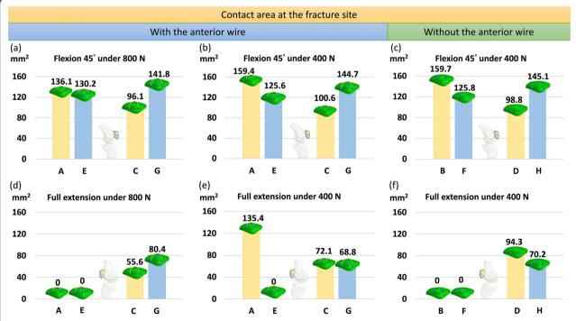
Fig. 8 Contact area between the fragments in knee flexion (a, b, and c) and extension (d, e, and f) under 800 N (left column) and 400 N (middle column) with the anterior wire and 400 N without the anterior wire (right column). Zero contact area meant that the two fragments are completely separated
