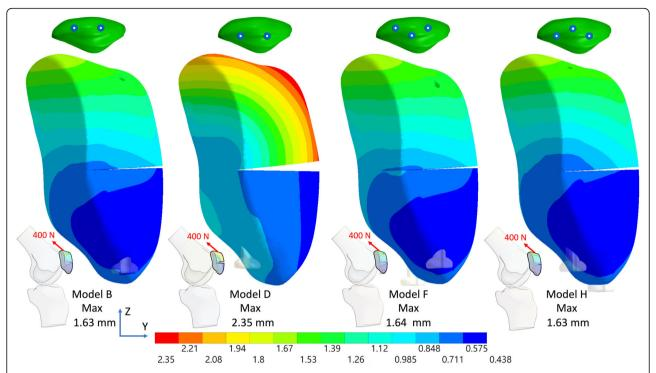
Fig. 5 Total displacement of the fractured patella with deep and superficial screws without the anterior wire plus the third screw in knee flexion 45° under a 400 N force. (Lateral view)
