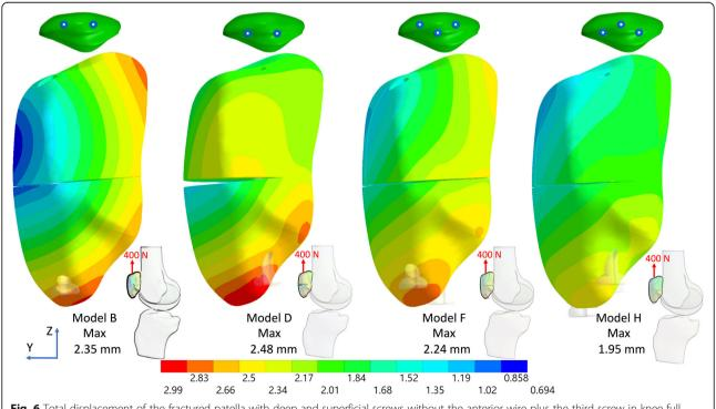
Fig. 6 Total displacement of the fractured patella with deep and superficial screws without the anterior wire plus the third screw in knee full extension under a 400 N force. (Medial view)
