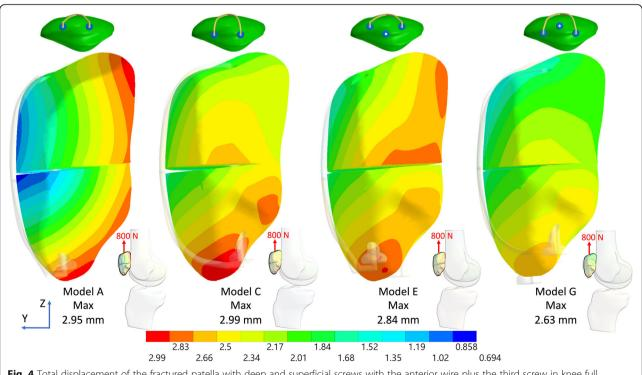
Fig. 4 Total displacement of the fractured patella with deep and superficial screws with the anterior wire plus the third screw in knee full extension under an 800 N force. (Medial view)
