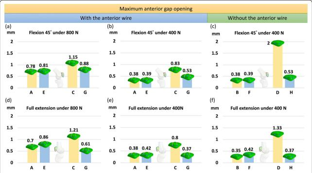
**Fig. 7** Gap opening distance in knee flexion ( $\mathbf{a}$ ,  $\mathbf{b}$ , and  $\mathbf{c}$ ) and extension ( $\mathbf{d}$ ,  $\mathbf{e}$ , and  $\mathbf{f}$ ) under 800 N (left column) and 400 N (middle column) with the anterior wire, and 400 N without the anterior wire (right column)
