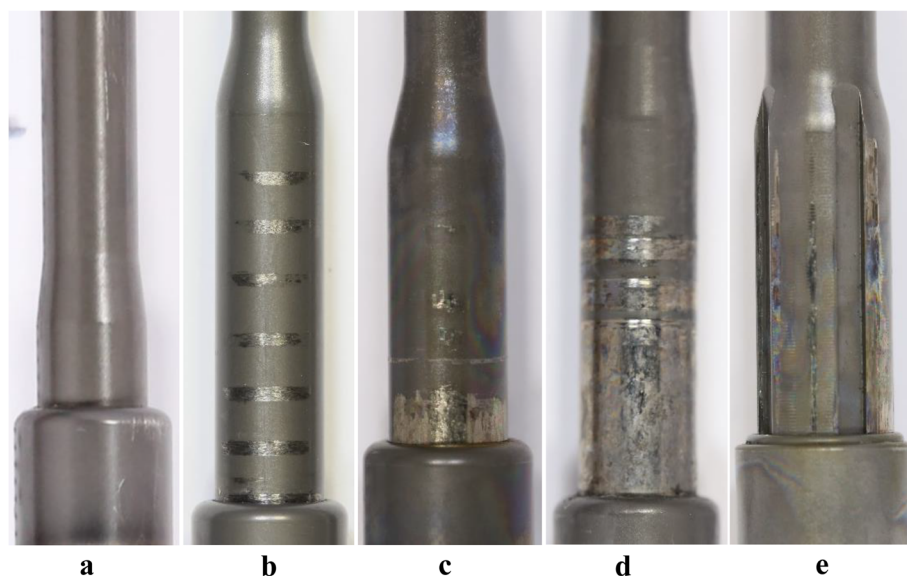
Fig. 6 Photographs of the telescopic region of five MAGEC rods showing no wear mark (a), circumferential wear marks (b), longitudinal wear marks (c), combined wear marks (d) and a modified telescopic design (e)
