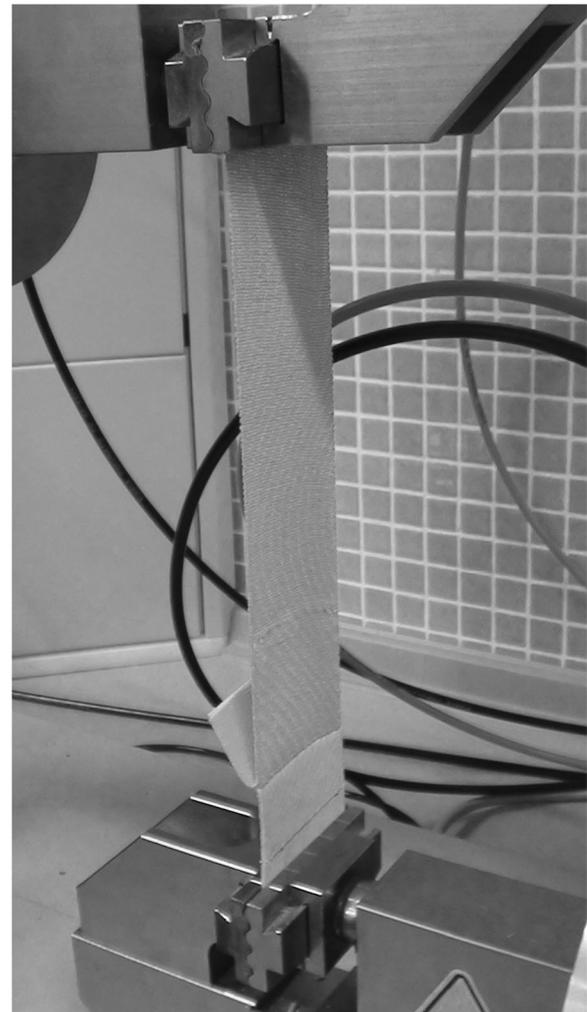
**Fig. 2** Dynamometer Zwick/Roell, model Z005 (Ulm, Germany) during the adherence test of one red tape. The tape is adhered on a piece of untanned sheepskin
