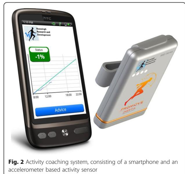
**Fig. 2** Activity coaching system, consisting of a smartphone and an accelerometer based activity sensor
