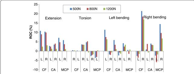
Fig. 12 ROC (rate of change) of facet contact force, contact area, mean contact pressure at the L4-L5 level in different loading conditions. L: left facet; R: right facet; CF: contact force; CA: contact area; MCP: mean contact pressure
