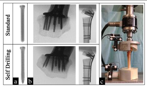
Fig. 2 Outline of the two groups, the screws used and the final setup. a) Individual screws; b) Tangential (skyline)- and lateral views of the prepared specimens; c) Biomechanical test-setup (mounted with only one container shell for illustration)
