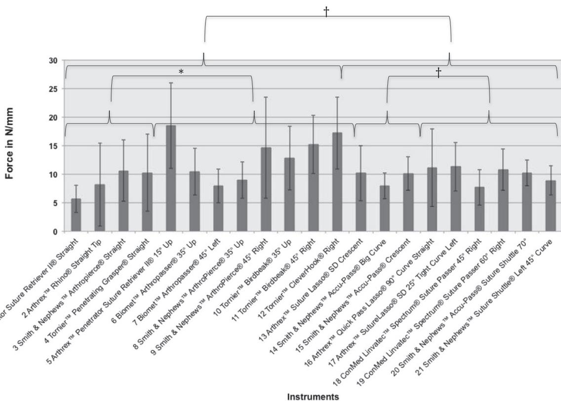
**Fig. 4** Mean values of all instruments in N/mm are shown. Brackets indicate statistical comparison. Suture Retrievers needed significantly more force to pierce the tendon than Suture Shuttles. The angled Suture Retrievers needed significantly more force to pierce the tendon than straight Suture Retrievers. There was no significant difference of straight and angled instruments within the group of Suture Shuttles. \*p = <0.05 † p = > 0.05
