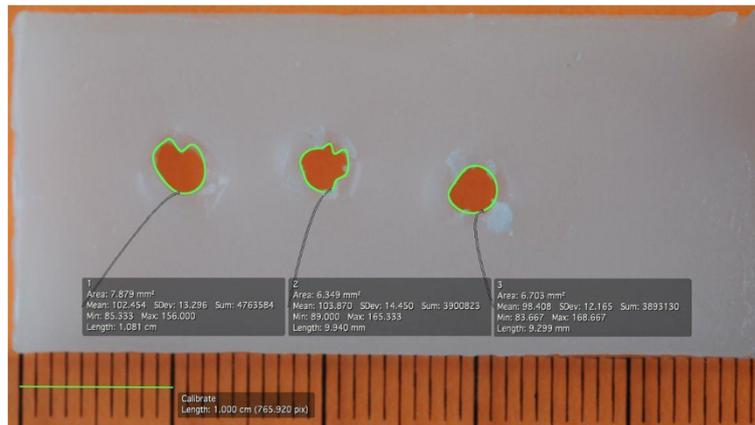
**Fig. 3** Software to measure the area in mm<sup>2</sup> of the three perforation marks, which were set with each instruments. Twenty-one bonewax plates were used and sixty-three values could be obtained. Values were compared looking at instrument function and type
