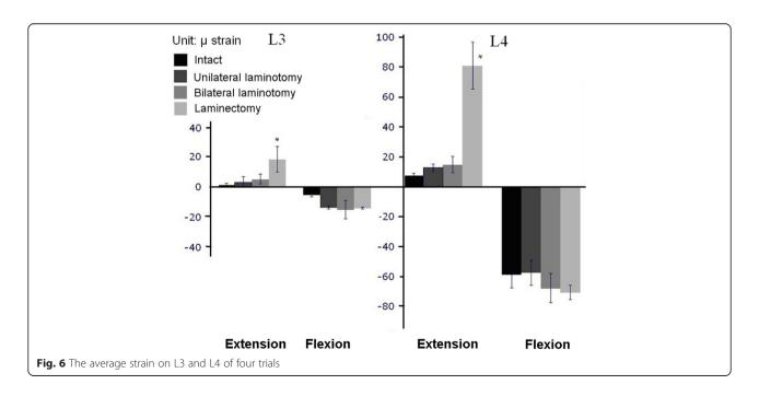
the intact group during flexion; by contrast, opposing results were found during extension. If either laminotomy or laminectomy involved removing the posterior elements of the spine, it would affect the extension more than the flexion. During extension, the posterior element plays a crucial role in stoppingany motion, like a stopper. Unilateral and bilateral laminotomies causing a higher degree of extension than that observed in the intact spines may be attributable to the aforementioned reason.
