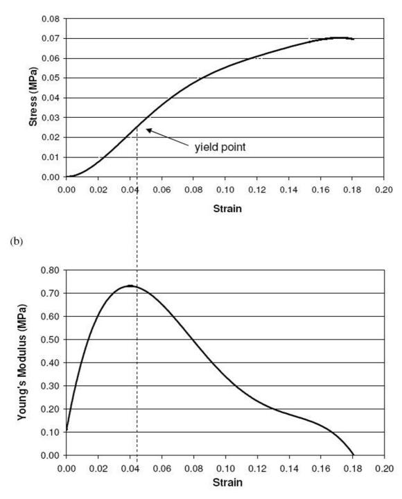
Figure I Stress-strain and Young's modulus-strain curves. (a) Stress-strain curve from a 7.7 mm length sample of open cell PU foam (0.09 g.cm<sup>-3</sup>) used to model very low density human cancellous bone and (b) the Young's modulus determined from it as the gradient of the curve. The yield point is defined by the point at which the Young's modulus decreases by 3% from its maximum value. The area under the stress-strain curve up to the yield point is defined as the energy absorbed to yield.
