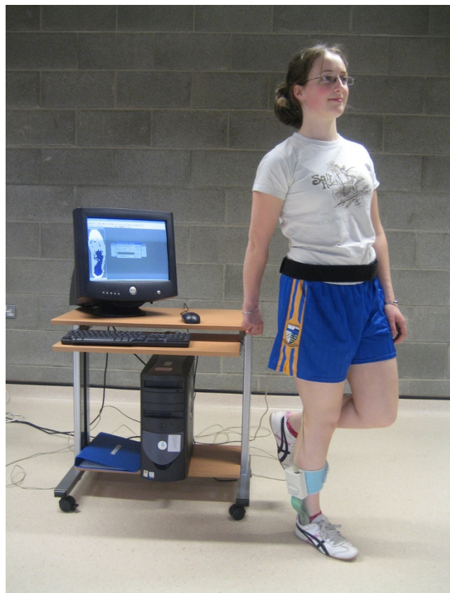
Figure 2 Calibration procedure for the F-scan plantar pressure system.
