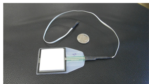
Figure 2 The FSR pressure sensor allowing to standardize the tension of the lumbar belts. To homogenize the pressure applied on the sensor, the 4.0 \times 4.0 cm sensor was supported with a semi-rigid plastic sheet and covered with a Styrofoam layer (total thickness of the three layers: 2 mm).
