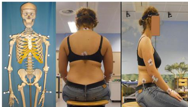
Figure 1 Skeletal model with markers and test person sitting on the chair, prepared with the markers for the 3D motion analysis using the HUX model.
