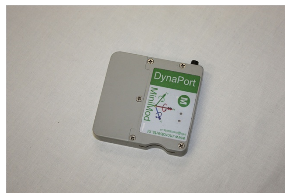
Figure 1 Three-dimensional gyroscope DynaPort MiniMod TriGyro ShoulderTest.
