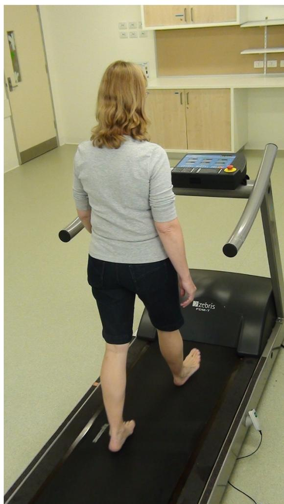
**Figure 1 Instrumented treadmill system.** Spatiotemporal gait parameters and ground reaction forces were estimated using an instrumented treadmill system that incorporated a capacitance-based pressure array consisting of 7,168 transducers with a spatial resolution of 0.85 cm.
