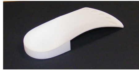
Figure 4 FO with adjustable metatarsal support elements. CAD model (left) and fabricated device (right). 2 nd to 4 th adjusters not shown in CAD model for clarity. Sections of the adjustable elements and their corresponding holes in the FO are threaded, allowing their height to be easily adjusted with a screwdriver.
