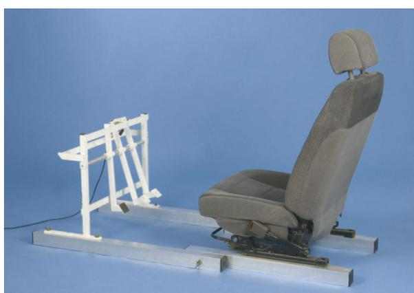
**Figure 2** Custom-made apparatus to measure brake response time.
