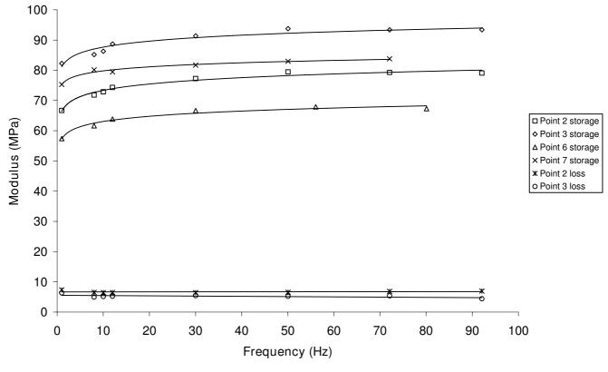
Figure 2 Storage and loss moduli against frequency, for frequencies of up to 92 Hz.
