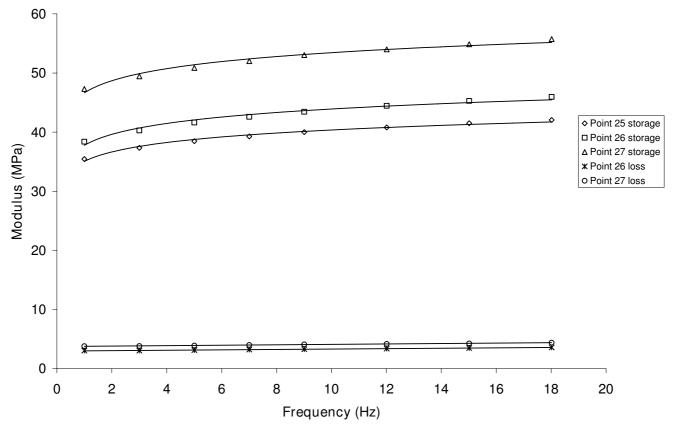
Figure 3 Storage and loss moduli against frequency, for frequencies of up to 18 Hz.
