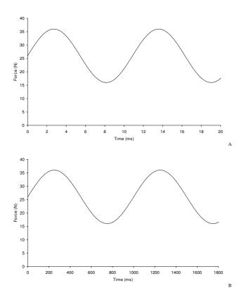
Figure I Sinusoidally varying force A) at 92 Hz (rise time 5.4 ms); B) at I Hz (rise time 500 ms).
