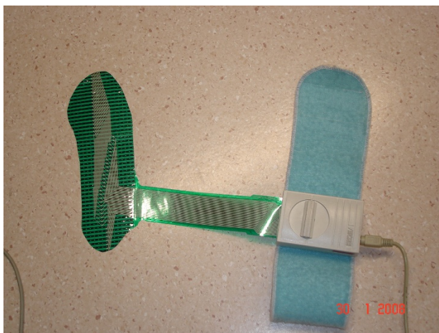
Figure 1 F-scan components – shown are the plastic insole, Velcro strap, cuff unit, and cable.
