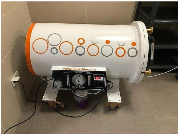
Fig. 1 Hyperbaric oxygen chamber designed for animals
