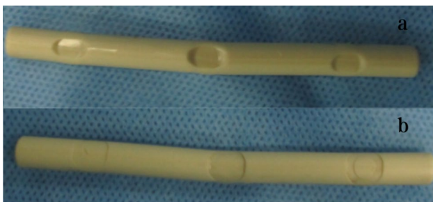
Fig. 4 Plastic indentation of retrieval PEEK rod on the nut (a) and screw (b) interface
