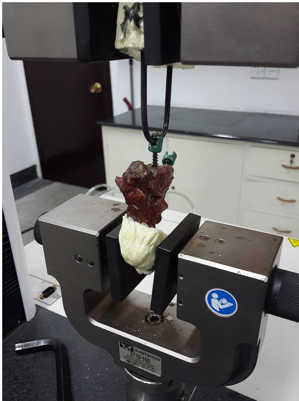
Fig. 2 Portrays the experimental configuration, whereby each specimen is individually secured in a pot and aligned with the cervical vertebral screw axis utilizing the Instron 8874 machine (Instron, Canton, Massachusetts)
