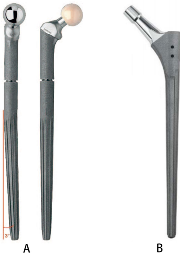
Fig. 1 A: Tapered fluted modular titanium stem (MP; Waldemar Link, Hamburg, Germany). The dentate structure in the proximal part of the prosthetic stem can bind with the tooth in the head and neck component. These two parts are fixed by screws. The surface of the prosthesis is covered with micropores of 70 microns, which is good for bone ingrowth. The distal end of the stem is tapered with a 3-degree curvature, which helps accommodate the bow of the patient's femur. The prominent crests on the surface increase the fixation of the distal femur. B: tapered fluted nonmodular titanium stem (WE-Cone; WeiGao, Weihai, China). The distal end of the stem is tapered with 8 crests to increase its anti-rotational stability
