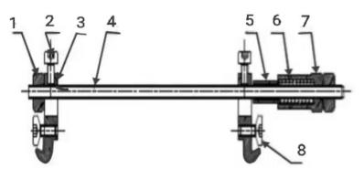
Fig. 1 Structure diagram of skin traction device. 1.limit nut, 2-limit screw, 3-fixing hook, 4-threaded rod, 5 -scale tube, 6-spring, 7-adjusting screw sleeve, 8-fixing pin screw
