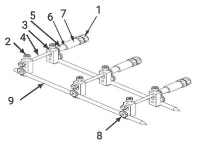
Fig. 2 Schematic diagram of skin traction device. 1-limit nut, 2-limit screw, 3-fixing hook, 4-threaded rod, 5-scale tube, 6-spring, 7-adjusting screw sleeve, 8-fixing pin screw, 9-traction pin
