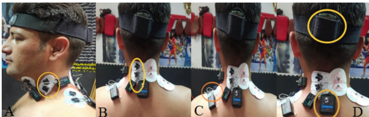
Fig. 1 Placing EMG electrodes (SCM: Fig A, ES: Fig B, UP: Fig C) and mounting IMU sensor (Fig D)
