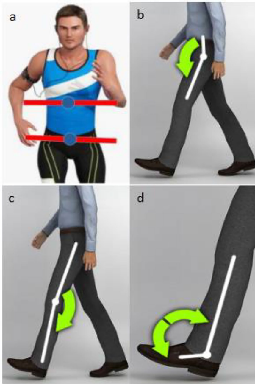
Fig. 2 a Trunk rotation ROM. b Hip flexion/extension ROM. c Knee flexion/extension ROM. d Ankle plantarflexion/dorsiflexion ROM. (from the STT motion capture system instruction manual)
