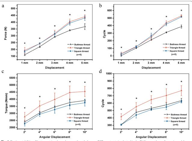
**Fig. 4** Fixation stabilities of buttress-, triangle- and square-threaded screw–DCP constructs implanted in the PU foam under cyclic craniocaudal loading (**a**, **b**) and cyclic torsional loading (**c**, **d**) of the foam block. (One-way ANOVA:  $*P \le 0.05$ )
