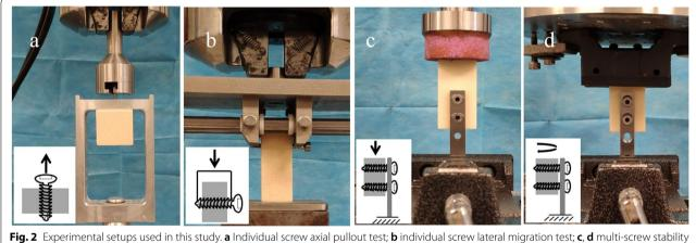
Fig. 2 Experimental setups used in this study. a Individual screw axial pullout test; b individual screw lateral migration test; c, d multi-screw stability of plate fixation test under craniocaudal loading c) and torsional loading d)
