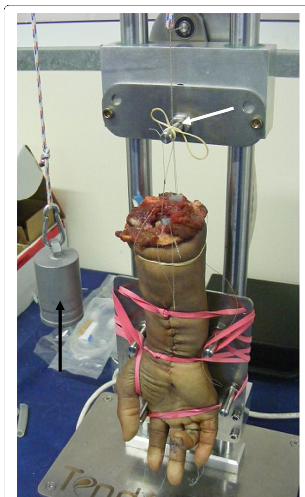
Fig. 4 Cyclic flexion–extension using the finger motion simulator. The hand is fixed to the device. The flexor tendons are tied to the motor that provides 2 cm tendon excursion (white arrow). The extensors are tied through a pulley to a 1 kg weight (black arrow) that allows straightening of the finger when the flexor load is removed
