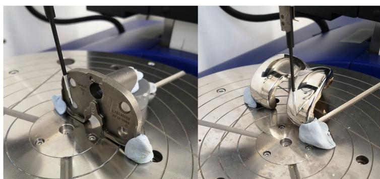
**Fig. 4** Example of surface roughness analysis performed using a contact profilometer
