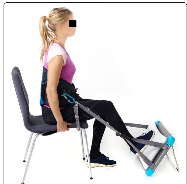
Fig. 2 Nintendo Wii Balance Board mounted to the aluminium frame and attached to the harness using straps, during isometric lower limb strength assessment
