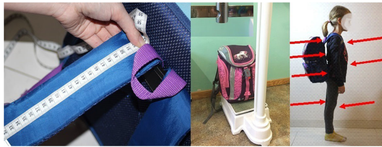
Fig. 1 The assessment of straps lengths, school bag's weight and school bags' positioning on pupils' back
