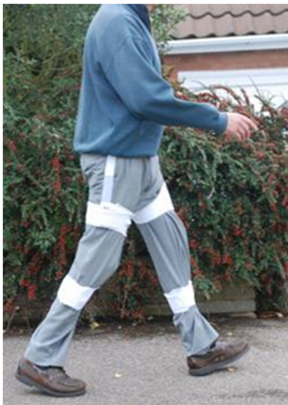
Figure 1 Volunteer walking with the IMUs strapped to the thigh and shank.
