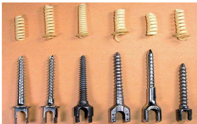
Figure 4 The spiral of bone chips. The spirals of bone chips were peeled from the surface of the screw threads.
