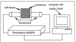
**Figure 1 Block diagram of QUS measurement system.** Two ultrasound transducers are fixed coaxially on both sides of the calcaneus and are coupled to the skin through coupling gel. Ultrasonic pulse is generated from one transducer, transmitting through the calcaneus and detected by another transducer. The detected signal is amplified by 5800 PR and output to GaGe CompuScope 12400, where the signal is sampled and converted to digital signal for further analysis.
