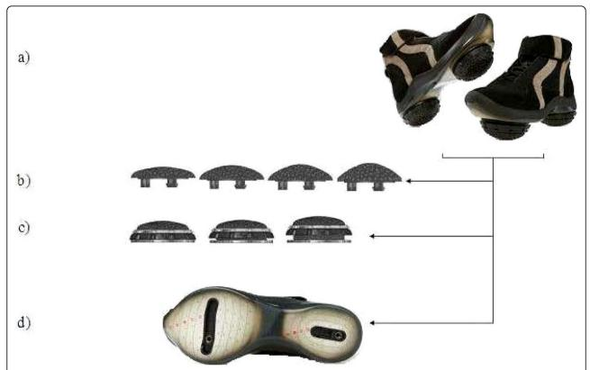
**Figure 2** The biomechanical device. (a) Bio-mechanical device comprising of two individually calibrated elements and a foot-worn platform which they are attached to under the hindfoot and forefoot regions. (b) Bio-mechanical elements are available in different degrees of convexity and resilience; (c) Height versatile base with 0.25 mm increments; (d) Specially designed sole includes two mounting rails and positioning matrix to enable flexible positioning of each bio-mechanical element.
