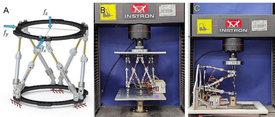
Fig. 3 The accuracy examination of the novel LS-measurement system. (A) Three types of linear test loads were applied. (B) Loading vertically to examine the accuracy along the z-axis. (C) Loading horizontally to examine the accuracy along the x-axis and y-axis
